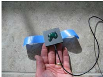
Figure 1: Heat flux sensor with conductive paste.
