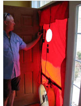
Figure 5. Blower door test.
